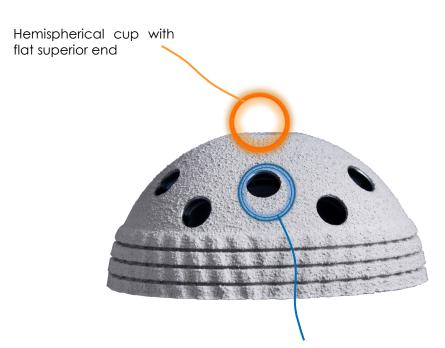
Upper quadrant of cup has 3 to 5 holes (depending on cup size) for Ø6.5 mm screws (available in lengths of 16 mm, 20 mm and then in 5 mm increments up to 45 mm)
