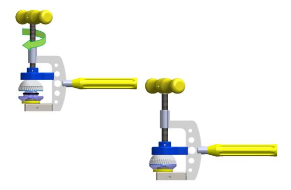
Take out the **HORIZON® II cup without hole** of the size validated by the trial cup. Remove the protective foam between the cup and its impaction plate.
