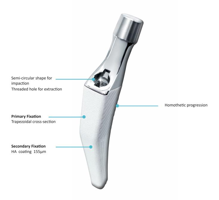
Material = Titanium alloy (Ti6Al4V)
