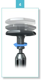
Keep the shaft with the strike plate in high position, so the thread end is retracted.
