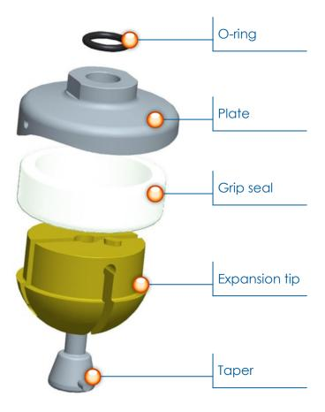
The plate and the expansion tip must be of the same size (check engraving on the instruments). The expansion tip must be correctly oriented compared to the plate : the peg of the expansion tip must fit inside the slot in the plate.
