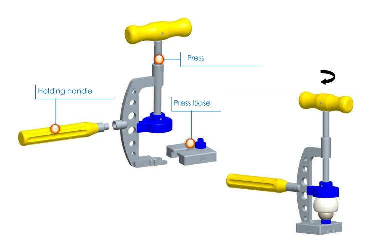
Secure the handle and the baseplate on the dual mobility cup press. Fully loosen the yellow T-handle.
